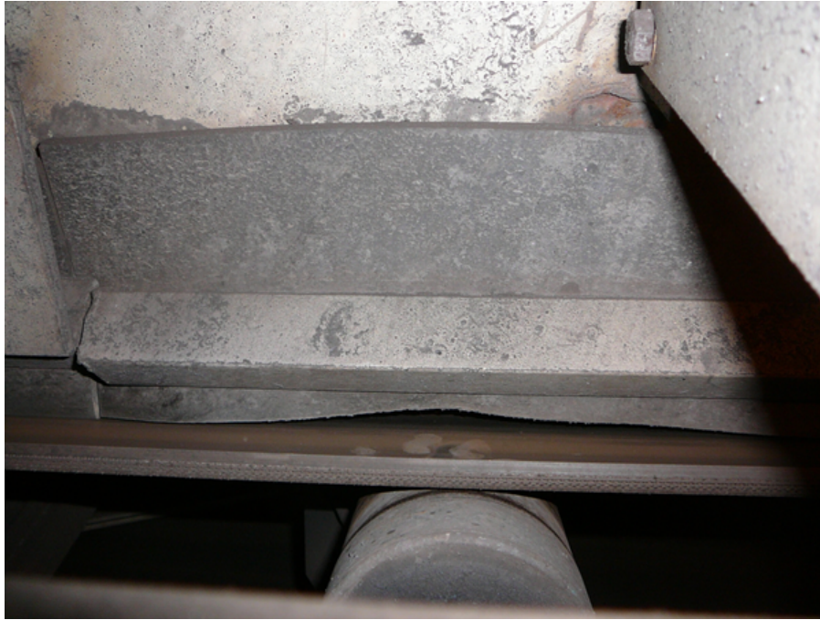
Crescent Shaped Wear Over Idlers Caused by Loading on the Transition or Excessive Belt Sag
