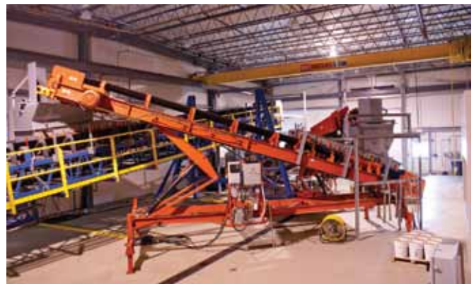
A three-part recirculating conveyor system at Martin's Center for Bulk Materials Handling Innovation allows for full-scale materials handling testing.
