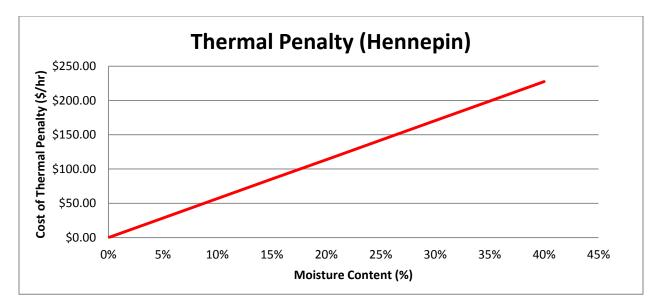
This facility receives coal at 37.37% entrained moisture. This facility loses  $\sim$ \$210 per hour just to dry out their coal.
