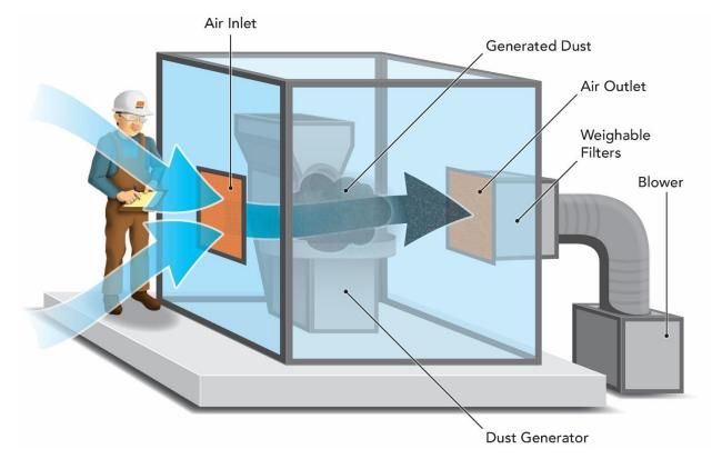
The blower and openings are sized large enough to capture all of the dust before it has a chance to settle, but not so large as to actually interfere with the material stream.
