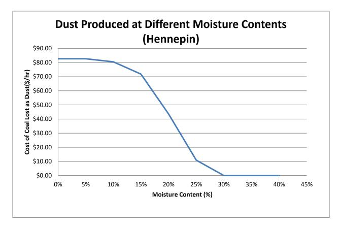
This graph shows that if this facility were to eliminate their dust entirely, they would save  $\sim$ \$80 per hour in lost material.
