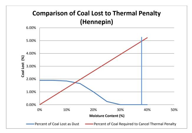
This shows that the coal comes in with 37.75% moisture entrained. The operation is already losing  $\sim$ 5% of its coal to correct for this. At this level of moisture, dust is not created anyway. It does not make sense for this company to add water at this point in the process assuming the moisture content remains at 37.75%
