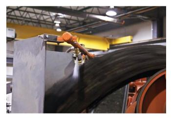
The unknown item was always the amount of water required to stop the dust from being generated. This amount of water required is based on the material properties and varies from application to application. Martin Engineering developed a test apparatus and procedure to determine the effect of moisture on potential created dust.
